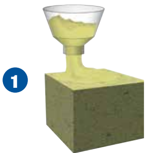
PENETRON ADMIX is added to the concrete at the time of batching.
