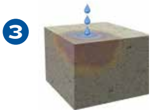
The crystalline technology is activated in the presence of moisture.
