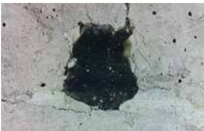
Close-up of a concrete cross-section showing the swelling properties of PENEBA SW waterstop.
